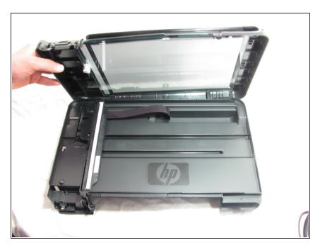
With the top half of the printer separated, lift the upper section with the scanner glass away from the lower section of the printer.
