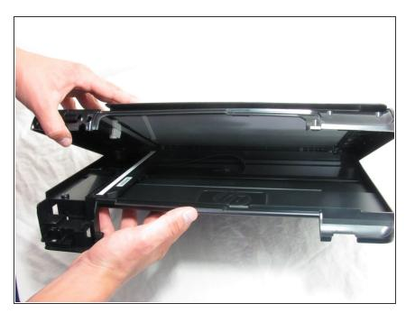
Pull the printer hood upward.
