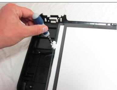
With the glass facing upwards, remove the screw holding the glass in place.
