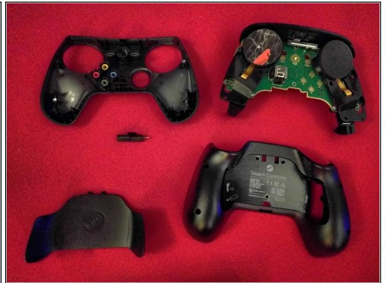
ⓘ I did not have a long enough screwdriver, so I ended up drilling out two of the four side screws.
