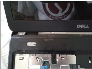
Use a plastic tool to separate the top of the laptop.
