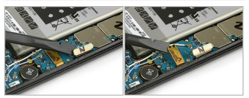
• Use the flat end of a spudger to disconnect both the display and the touchscreen cables.
