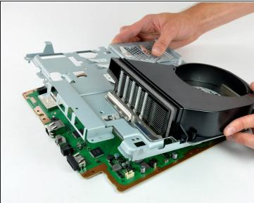
• Separating the metal electromagnetic interference shield from the logic board.
