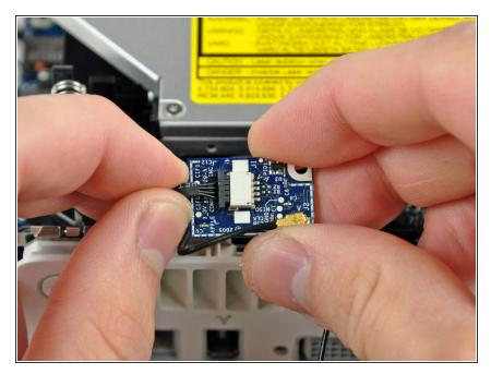
Disconnect the Bluetooth cable connector by pulling it straight away from its socket.
