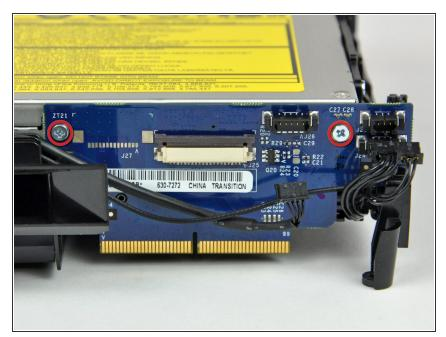
Remove the two Phillips screws securing the interconnect board to the optical drive.
