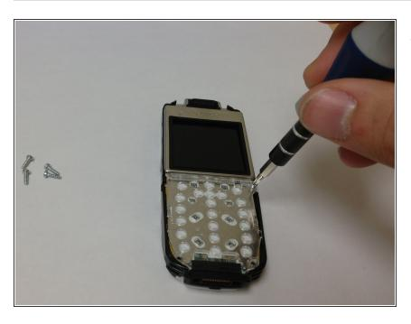
Use a T5 Screwdriver and unscrew the five screws.
