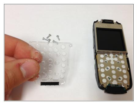
Once the screws are off, there should be a plastic cover on top of your screen. Gently slide the plastic cover off.
