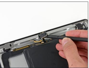
• Use the flat end of a spudger to pry the camera ribbon cable out of its socket in the plastic antenna housing.
