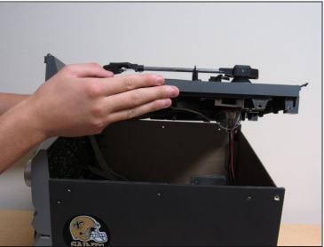
• Lift the base that the turntable was resting on from the rest of the device.
