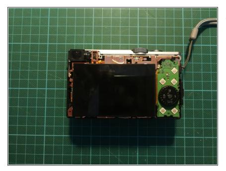
The backbody is lose now, remove it carefully and it reveals the controls and the display
