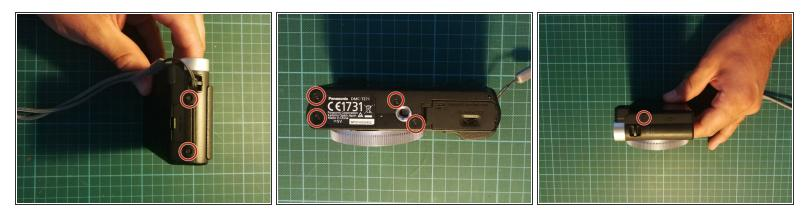
• Open all 7 screws with a fitting philips screwdriver.
