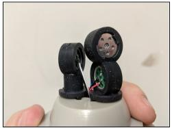
• As seen in the picture, this Microphone cap comes with a internal foam guard to protect the three internal mic condensers. These point outward to the side of the mic making this mic more useful from the side and not pointed at the users itself.
