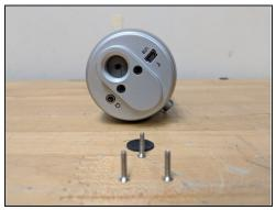
• First remove the Rubber inside the screwable mount area. This can easily be done with a small screw driver tip or <u>Tweezers</u>. From here you can remove the 3 screws using a #1 Phillips head.
