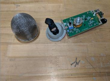
• If you look toward the mesh and the circuits you will see that it is held by 4x #0 Phillips screws. Carefully remove these and the entire cap will come from the board. There are 3 sets of wires, 1 per condenser. You will notice that they are pointed sideways, making this microphone a side condenser, not a face-pointed one.
