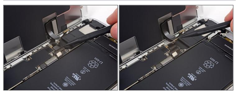
Disconnect the second lower display cable connector, directly behind the one you disconnected in the previous step.
