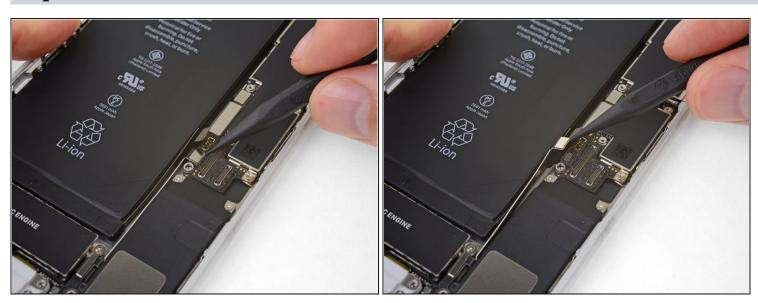
Use the point of a spudger to pry up and disconnect the antenna flex cable from the logic board.
