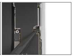
Use the point of a spudger to push the SIM card eject plunger out of the logic board's way.
