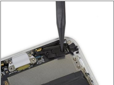
• Gently push the barometric vent in the direction of the battery to separate the adhesive securing the vent to the bottom edge of the iPhone.
