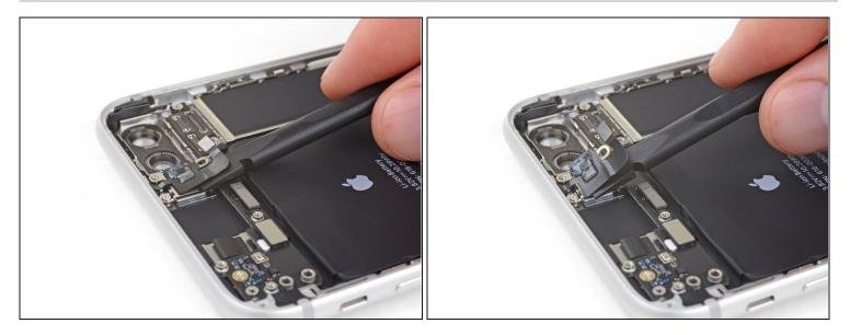
• Slide the flat edge of a spudger underneath the antenna flex cable to separate the adhesive holding it in place.
