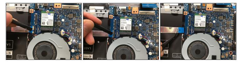
• Use the tip of a spudger to flip up the retaining flap on the daughterboard ribbon cable ZIF socket on the motherboard.
