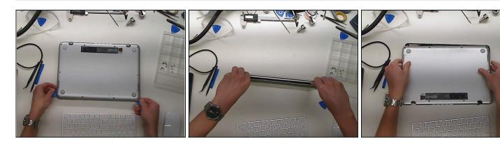
Use a plastic pry tool to get in-between the bottom cover and the lower case assembly.
