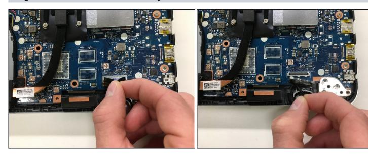
• Pull straight up to disconnect the display cable
