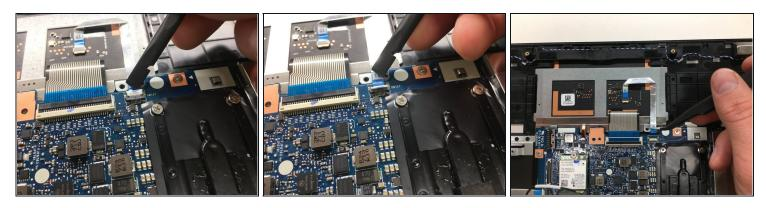
• Use a spudger to flip up the retaining flap on the trackpad ribbon cable ZIP socket.
