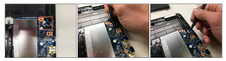
Use a Spudger to push the left speaker cable out the connector.
