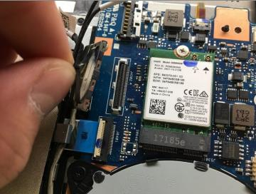
• Pull straight up to disconnect the SATA combo cable from the motherboard.
