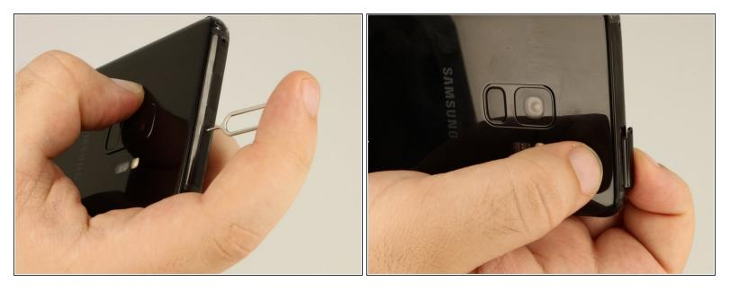
The SIM card tray's ejection hole and the microphone hole look very similar, be very careful not to insert the tool inside the microphone hole or you might damage the microphone.
