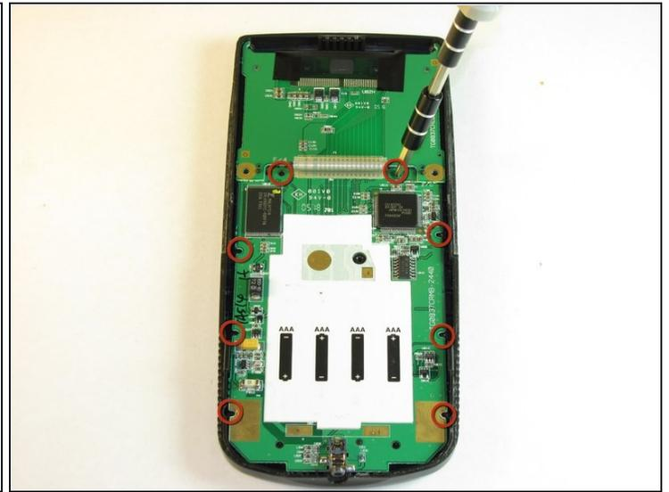
ⓘ Keep the screen face-down during this step. Only the motherboard is attached to the face-plate and the screen may fall out.
