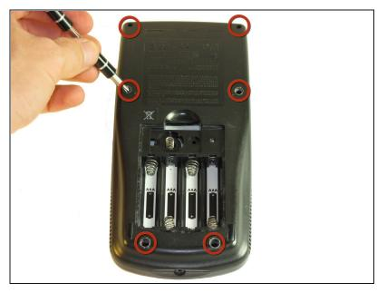
Unscrew the six 7.5mm T6 screws on the back case. You will need to use a screwdriver with a long and skinny head.
