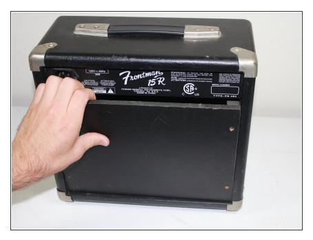
Once the top is separated, use your hand to remove the back panel from the unit.
