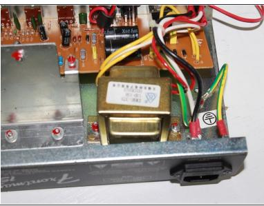
Locate the transformer on the metal mounting bracket and be sure that it looks the same as the replacement that you plan on installing.
