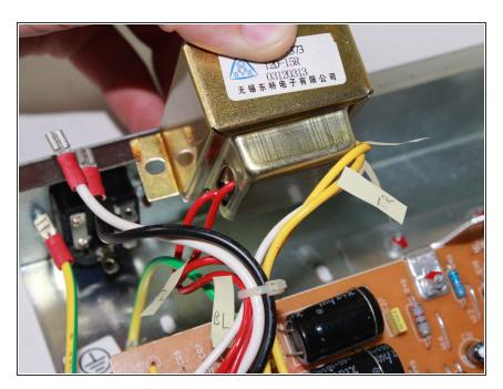
Label, make note of, or memorize the arrangement of all wires going to and from from the transformer.
