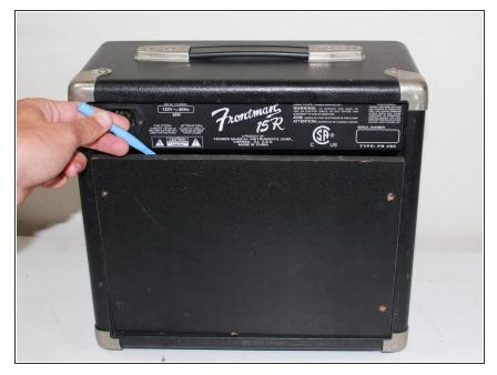
Once the screws are out, use a plastic opening tool or spudger to pry the top of the back panel open.
