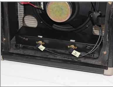
There will be two black wires connecting the top mounting bracket to the reverb box at the bottom of the unit. Label the wires to prevent crossing upon re-installation, then unplug the wires from the reverb box.
