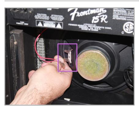
Label and unplug the two red wires connecting the mounting bracket to the speaker by pulling them off the nodes.
