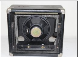
Pull the mounting bracket free from the frame. It may be wedged in very snug, in which case, use a
