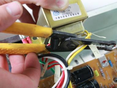
• Using wire cutters, cut the wires from the existing transformer leaving only enough wire next to the transformer to see the color of each cut wire. Then remove the transformer.
