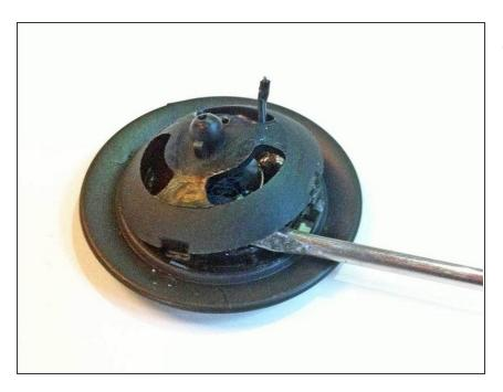
• Carefully remove the plastic cover with a flat screwdriver.
