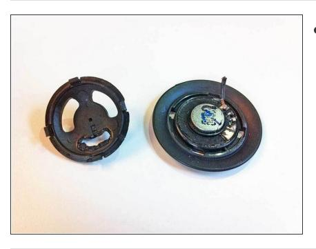
Redo the welds and reassemble the headset.
