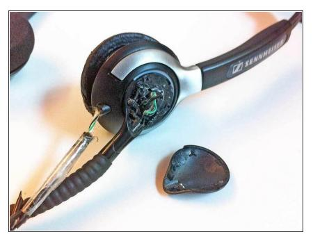
Carefully remove the plastic cap using a flat screwdriver or a thin spudger.
