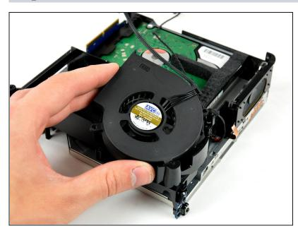
• Lift the fan out of the internal frame, minding any cables that may get caught.
