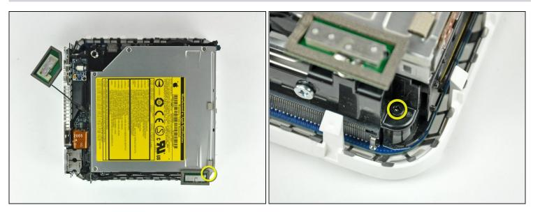
• Remove the Phillips screw from the internal frame near the Bluetooth antenna.
