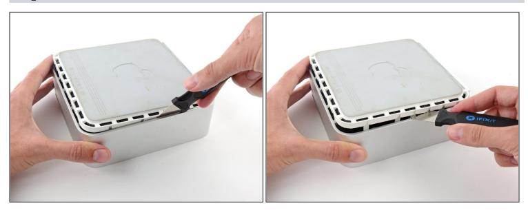
• Keep working around the perimeter, freeing the clips along the final edge.
