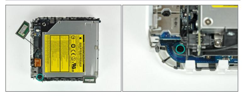
• Remove the Phillips screw near the audio ports securing the internal frame to the bottom case.
