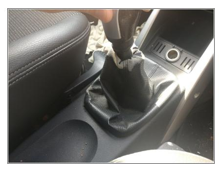
Examine existing gaiter and take note of how its installed. A quick snap with your camera phone is helpful!
