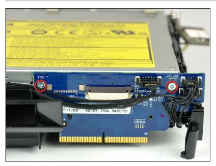
Remove the two Phillips screws securing the interconnect board to the optical drive.
