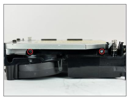
Turn the mini 180 degrees and remove the two Phillips screws securing the optical drive to the internal frame on the other side.
