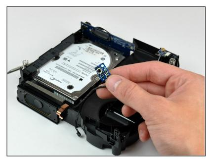
De-route the IR board and cable through the channel near the hard drive in the internal frame.
