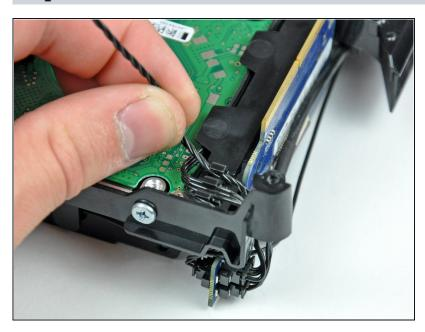
De-route the IR board and cable through the small plastic clip in the internal frame.
