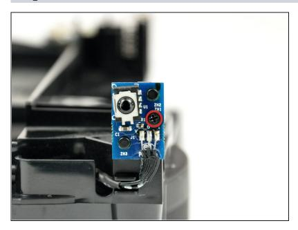
Remove the single Phillips screw securing the IR board to the internal frame.
