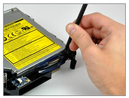
Use the flat end of a spudger to separate the interconnect board from the optical drive.
