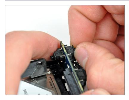
Use your fingers to disconnect the IR cable connector from its socket on the interconnect board. Make sure to pull straight out, and to pull on the connector and not the cable.
