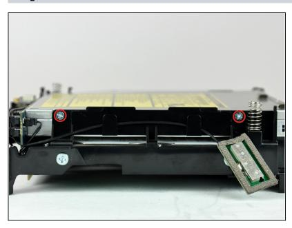
Remove the two Phillips screws securing the optical drive to the internal frame.
