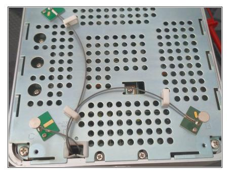
Take care not to damage the wires of the Wi-Fi antennas which are very bothersome.
