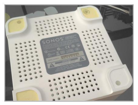
Remove the rubber pads and unscrew
