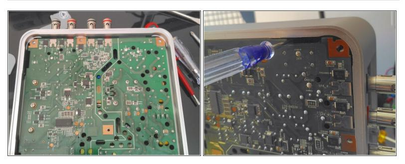
By using a screwdriver inserted through each of the 8 peripheral slots, you can access the clips of the top cover.
