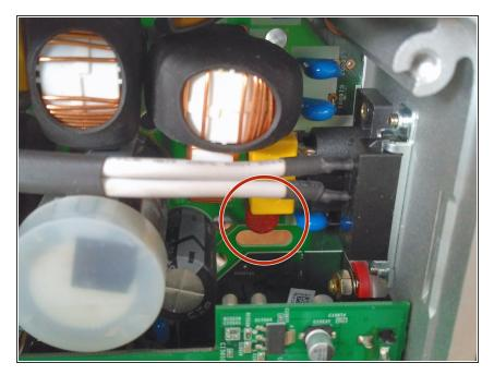
It's a soldered fuse. You will need to desolder it from the back in order to replace it.
