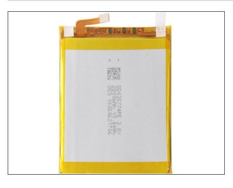
Insert new battery. You may wish to stick it down with the new white strips. To reassemble your device, follow these instructions in reverse order. Make sure the two buttons are inserted in the frame the right way around when reassembling.
