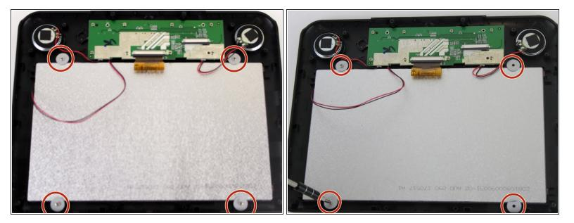
Unscrew the corners of screen with the JIS #000 screwdriver. There are four, 6 mm screws with washers.
