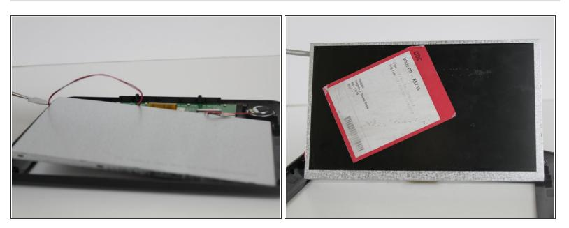
After the screws and washers are removed, you can lift the screen off with the pry tool.
