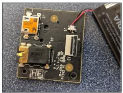
• From here you can remove the Single Phillips Screw using the Phillips 00 Driver Bit. This will let you pry the circuit and battery from the Glue. You can lift the Battery from the Circuit board as it is made to lift upward and away from the board.
