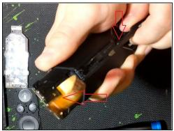
• The Sensor Ribbon is carefully peeled away from the glue. There are two options available to get the battery compartment out. You can either use the <u>Tweezers</u> and push near the ribbon cable or you can use the tweezers to push from the other end inside and under the Sensor place as seen in the picture.
