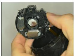
• You can see the two magnets, that are used to move the lens
