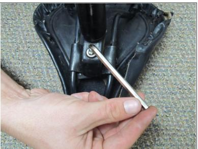
Use an Allen wrench to unscrew the bolt that is holding the post to the seat cushion.
