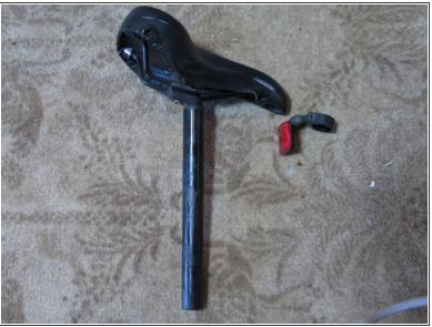
Now that the seat is loosened, slowly pull up on the seat cushion until it is fully out of the frame.
