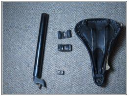
Now that the bolt is loosened, carefully pull the seat cushion from the post. Next remove the two riders as shown in the second image.
