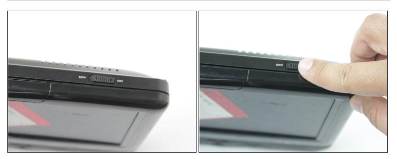
Turn the power off. Slide the power button to OFF.
