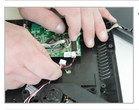
Once you have it loose, unplug it from the PC Board. Then the disk reader can be removed.
