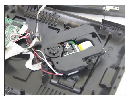
Locate the disk reader, it will be right under the disk chamber.
