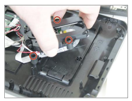
Pick it straight up, it should slide off the three pegs holding it in place, if not, wiggle each peg individually.
