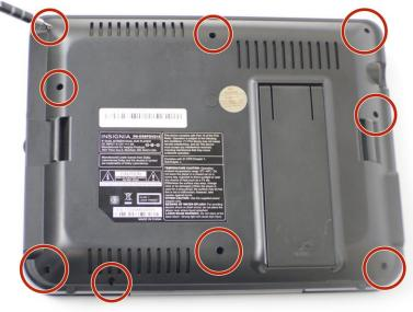
• Unscrew the nine 9mm screws with a JIS #000 screwdriver.
