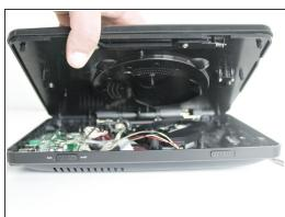
Pry off back panel with prying tool, then remove by hand.
