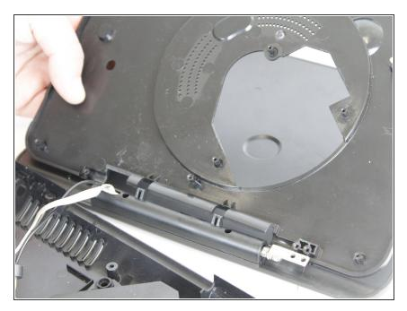
Slide the tray up and off of the hinge completely.
