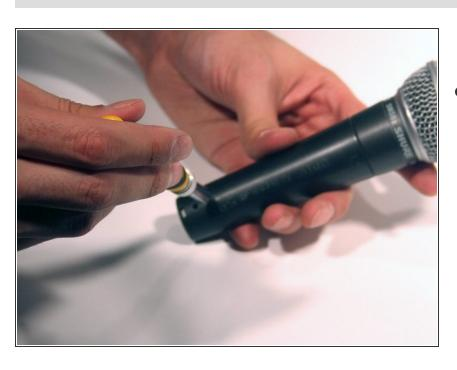
Using a small flat head screw driver, turn the screw in the side of the microphone clockwise until it is tight. Following these steps should reinstall the XLR connector back into the microphone.
