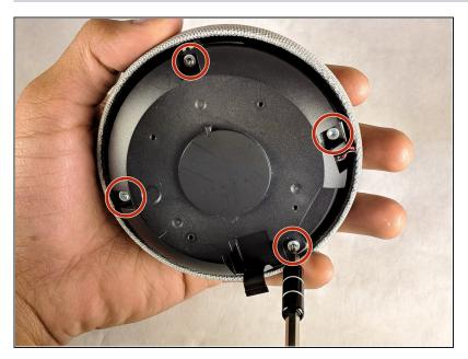
• Remove the four 7.8mm T8 Torx screws.
