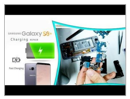
This tutorial will help you to resolve the matter with no charging or no connection to the PC. In order to replace the charging port follow the guide.
