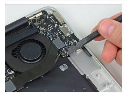
Use the edge of a spudger to pry the microphone connector up and out of its socket on the I/O board.
