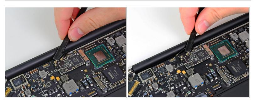
Use the flat end of a spudger to pry both antenna connectors up from their sockets on the AirPort/Bluetooth card.
