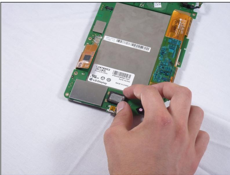
**⚠ When replacing the motherboard make sure that the speaker assembly component (small rectangular piece) is in place. It is not attached and needs to be properly aligned.**
