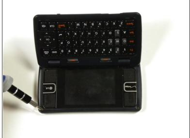
Use a Phillips #00 screwdriver to remove two 2.5 mm screws.
