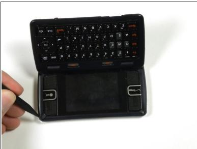
Use a spudger to pry the two rubber covers out of the device.
