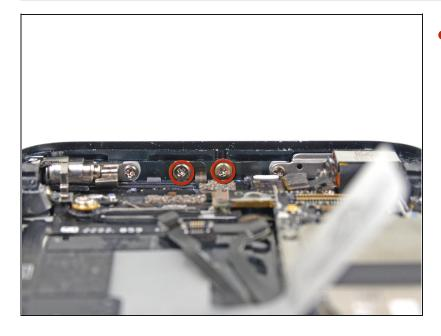
Phillips screws from the inner top of the rear case.
