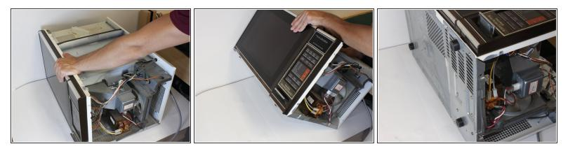
• Tip the microwave back so it is lying face up. This allows access to the screws beneath the transformer.
