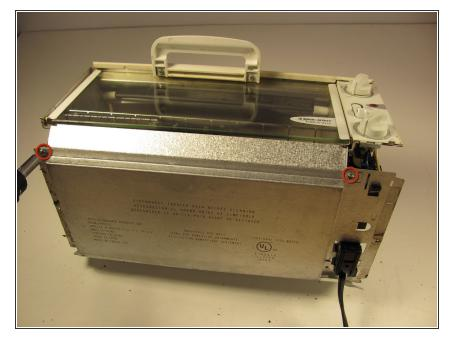
Remove the two Phillips #4 1 cm screws, which connect the bottom panel to the unit.
