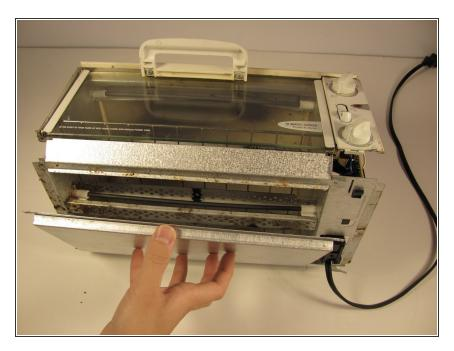
Remove the crumb tray (the bottom, metal panel) from the toaster unit.
