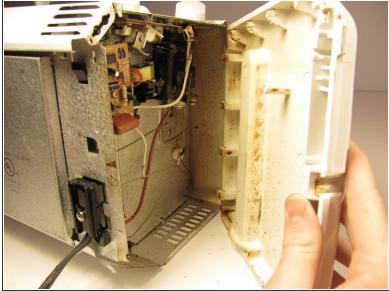
Pull downwards (towards the bottom of the unit) and outward to remove the side panels.
