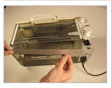
Remove the aluminum strip from the bottom of unit; this is the piece that is directly under the door.
