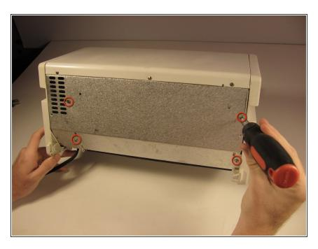
Remove the four Phillips #4 1 cm screws from the back of the unit.
