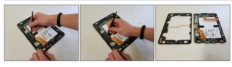
• Locate the ribbon running from the midframe and disconnect it from the motherboard with the flat end of a **spudger**.
