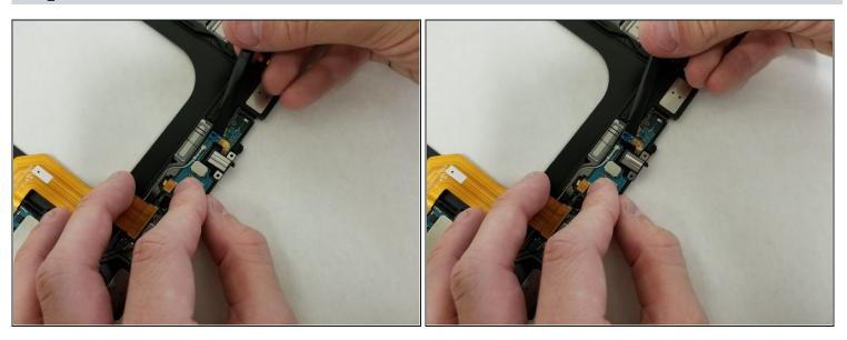
• Use the flat end of the **spudger** to snap the ribbon connector off of the motherboard.
