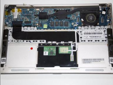
Disconnect fan from motherboard by pulling the small white and blue connector from its socket.
