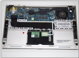
Remove the plastic piece (labeled M3 10) sitting on top of the fan by lifting from one edge and peeling it over.
