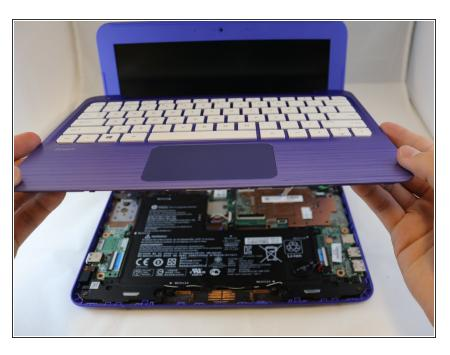
After detaching the two large ribbon cables, carefully lean the keyboard against the screen. To reassemble your device, follow these instructions in reverse order.
