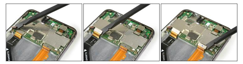
• Use a spudger to disconnect the volume and power button, the display and the main flex cable.
