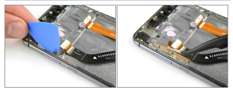
• Use an opening pick to cut the adhesive between the volume and power button flex cable and the mid frame.
