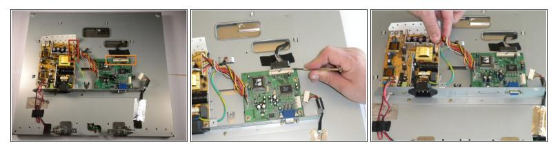
$\bigwedge$  Use caution when removing the connectors as they can easily break when removing.
