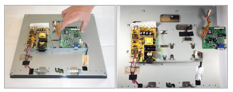
• Lift the motherboard straight up to remove it from the back panel.
