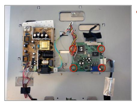
Remove the four 6.4mm #2 Phillips screws from the corners of the motherboard with a #2 Phillips screwdriver.
