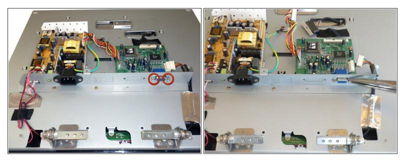
Remove the two 3/16" hex head screws from the VGA connecter. Use a pair of needle nose pliers
