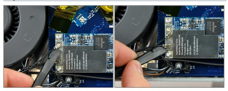
• Use the flat end of a spudger to pry both antenna cable connectors up off the AirPort card.
