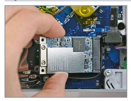
Pull the AirPort card away from its socket on the logic board.
