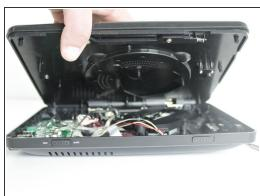
Pry off back panel with prying tool, then remove by hand.
