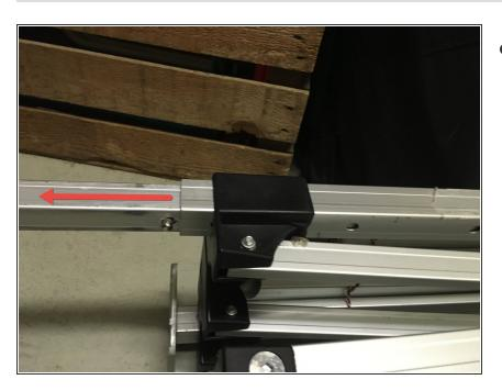
Pull the foot support out of the support leg.
