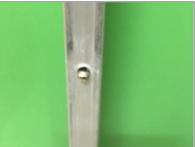
When the spring appears in the hole, continue to push gently until the bolt pops into the hole.
