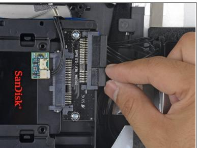
Connect the iMac's SATA data cable to the enclosure's SATA data connector.
