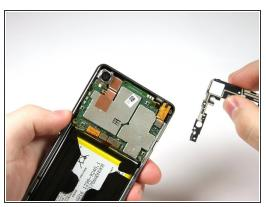
Pry up the black camera case with the plastic opening tool and then remove the case.
