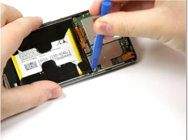
• Pop off the small connector on the right side of the motherboard with the plastic opening tool.
