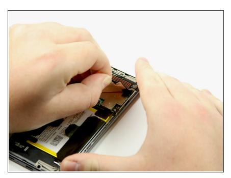
Peel back the RAF antenna.
