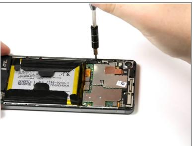
Remove the five black 4mm screws with a Phillips #00 Screwdriver.
