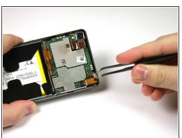
Pull out the square shaped connector using tweezers.
