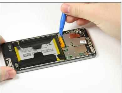
Pry up the copper connector next to the battery with the plastic opening tool.
