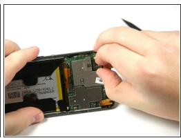
Pry up the camera's connector to the motherboard with the nylon spudger.
