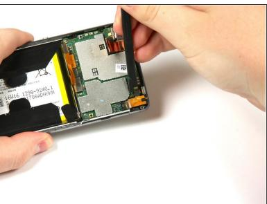
• Use the spudger to loosen the black connector from the top right of the motherboard.
