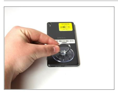
Stick the small suction cup on the bottom half of the back surface of the phone.
